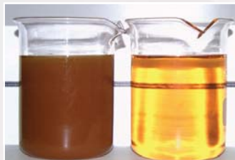
Turbine oil, before and after filtration
